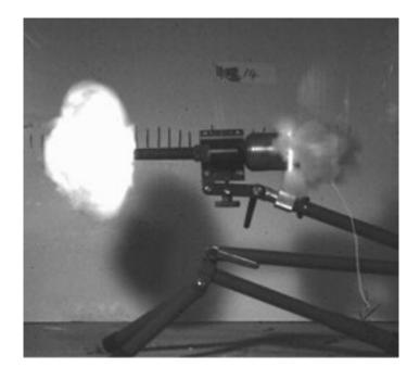
The disruptor is powered by an electrically initiated 12 gauge cartridge and features a 19mm bore barrel. The RE12g Mini Disruptor can be fired either electrically or by non-electric (percussive) shock tube.
