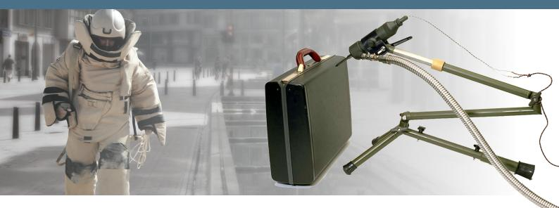
The Freeze Neutralising Kit (FNK) is designed to remotely deliver liquid nitrogen into threat packages to temporarily neutralise the power source. This gives the EOD technician a safety window for a safer disruption shot, or if the package is not defeated, will improve the recovery of material for forensic analysis.
