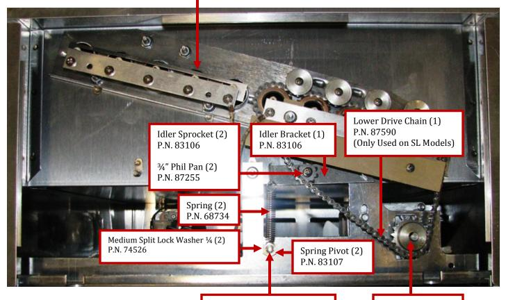
1/4 - 20 x 1/2 Hex Head Bolt (2) P.N. 14821 Sprocket Drive (2) P.N. 87353
