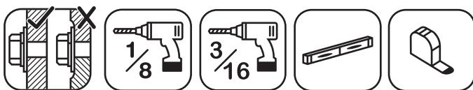
Pre-drill each hole using a 3/16" drill bit for WL5.
