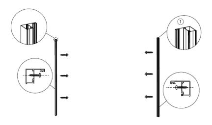
Step 3:Insert the zipper with fabric into the plastic zipper guide insert rails and align it to the side rail .
