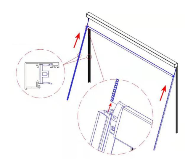
Step 4: Assemble the front rail tight by pushing the front rail into the back rail (while the plastic zipper guide insert is within).
