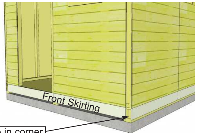
Gap in corner
