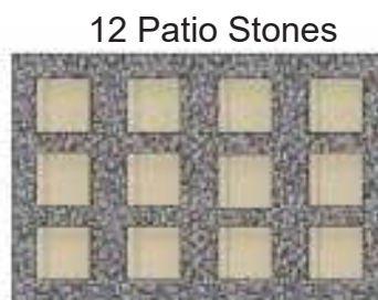
Gravel Foundation with Patio Pavers
