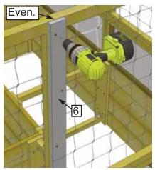
**9.** Position and attach short Vertical Panel Support using **3 - 2" screws** as **per Step 8.** Complete remaining rear and side walls.
