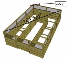
**1.** Prior to installing your Deer Fence Option Kit, confirm your 8x12 Raised Bed is level and square. Measure diagonally inside corner to corner (approximately 164 1/4") in both directions. Adjust as required. Use a level to determine if the tops of the bed frames are sloped and adjust if necessary.
