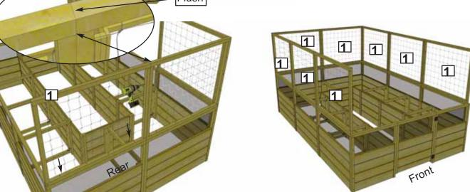
**4.** Position a second **Rear Panel (1) - 46" wide x 33 5/8" high** on top of the rear raised bed frame. Hold both rear deer fence frames together and starting at the top, screw together with 4 - 2 1/2" screws as shown above. Screw bottom of frame down to raised bed frame with 4 - 2 1/2" screws. Complete remaining side and rear panels attachments following Steps 2 and 3.
