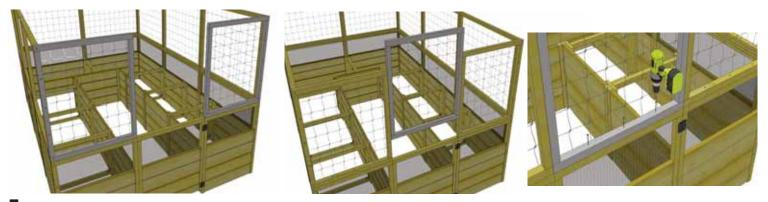
5. Locate all three Front Deer Fence Panels (2) - 30 5/8" wide x 33 1/2" high. Designate one to be a door panel and leave to the side. Attach both outside panels as per Steps 1 - 3 except use only 3 - 2 1/2" screws to attach bottom frame. Position and install designated door panel between front panels and screw only from bottom frame into top of raised bed door frame with 3 - 2 1/2" screws as shown above.
