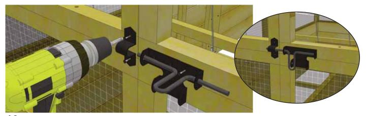
**10.** Attach Black Barrel Bolt to door and panel frame using **6 - 3/4" black screws**. Note how female part of Barrel Bolt is positioned higher than male. Do a dry run first to position Barrel Bolt correctly, then attach. Pre-drill with 1/8" drill bit to prevent wood from splitting.
