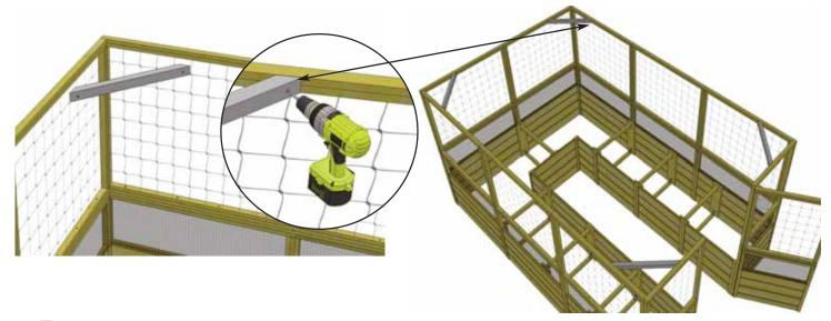
7. Attach Corner Brackets with angle cut ends - (4) on the inside frames at the top. Use 2 - 2 1/2" screws per bracket. Screw on an angle. Pre-drill ends with 1/8" drill bit to prevent wood splitting.
