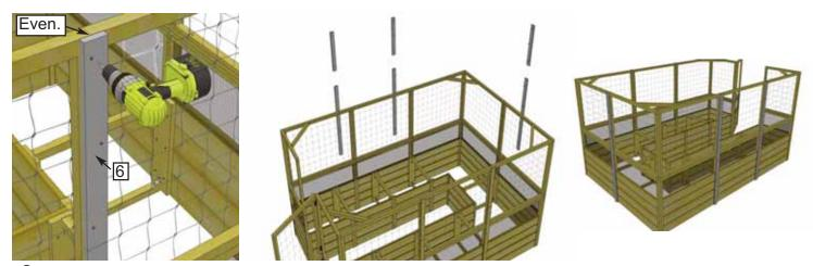
**9.** Position and attach short Vertical Panel Support using **3 - 2" screws** as **per Step 7**. Complete remaining rear and side walls.
