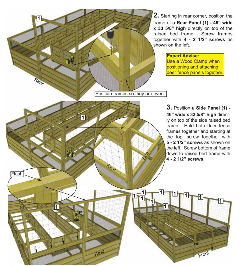
**4.** Position a second Rear Panel (1) - 46" wide x 33 5/8" high on top of the rear raised bed frame. Hold both rear deer fence frames together and starting at the top, screw together with 4 - 2 1/2" screws as shown above. Screw bottom of frame down to raised bed frame with 4 - 2 1/2" screws. Complete remaining side and rear panels attachments following Steps 2 and 3.
