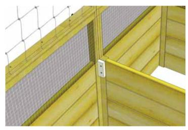
**11.** The **Door Stop (I)** and screws were included with your 8x16 Raised Garden Bed Kit. See **Step 21** of that manual. Install the Door Stop at the top of interior panel frame as shown above.
