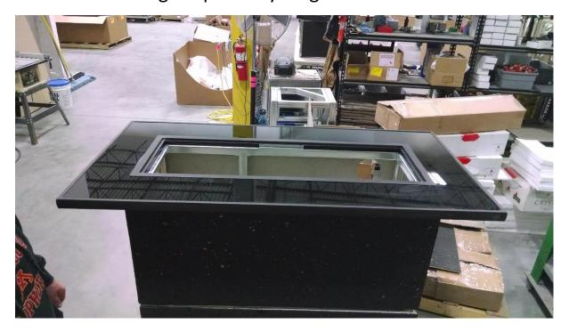
**5.** Using the remaining 4 #8-1/2" Phillips head self-tapping screws, secure Montego top to Key Largo base.
