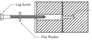
Before mounting Lag Screw, use factory drilled holes as guides to drill 1/8" pilot holes
