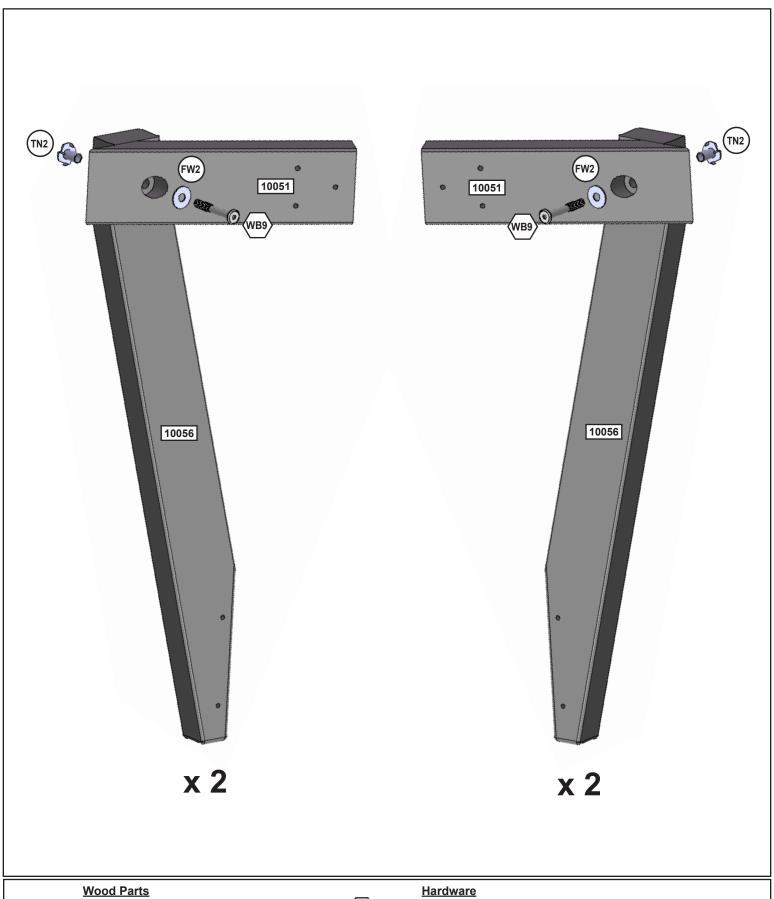
4 x 10051 31.8 x 76.2 x 263.0 mm (1-1/4 x 3 x 10-3/8") 4 x 10056 31.8 x 76.2 x 654.1 mm (1-1/4 x 3 x 25-3/4") Hardware 4 x wb9 7.9 x 54 mm (5/16 x 2-1/8") (FW2, TN2)
