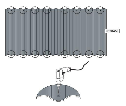
Pre-drill each hole using a 1/8" drill bit.
