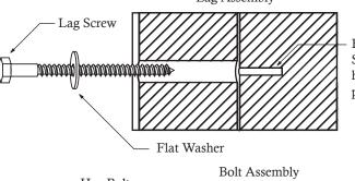
Before mounting Lag Screw, use factory drilled holes as guides to drill 1/8" pilot holes
