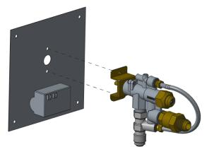
Attach burner valve to control panel with provided screws as shown below. Ensure sparker box is installed before this step.
