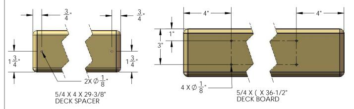
2: PLACE THE 5/4 X 4 X 29-3/8" DECK SPACERS BETWEEN THE CORNER POSTS. MAKE EACH DECK SPACER FLUSH TO THE INSIDE SURFACE OF THE 2 X 6. ATTACH EACH DECK SPACER TO THE DECK SUPPORTS WITH TWO 2" WOOD SCREWS. NOTE THE TOP OF THE SCREW HEAD SHOULD BE FLUSH WITH THE TOP OF THE DECK SPACER.
