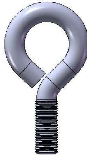
3/8"-16 X 3/4" DIA. I.D. X 2-1/2" L EYE BOLT QTY: 2
