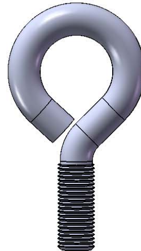
3/8"-16 X 3/4" DIA. I.D. X 2-1/2" L EYE BOLT QTY: 2
