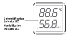
Humidification Indicator LED: If humidity Control Function selected humidification mode, the indicator LED is on, otherwise off.
