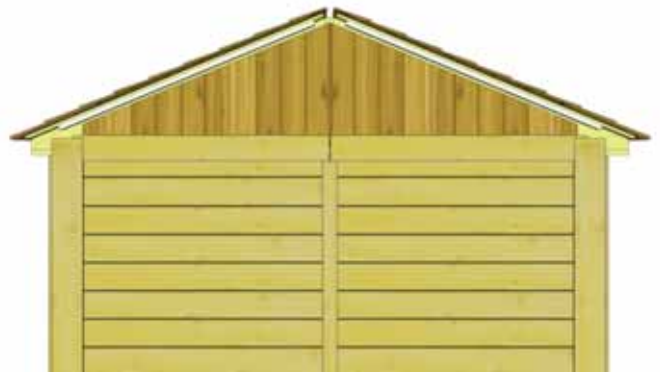
Facia/Roof Nailing Strips (4 @ 3/4" x 2 1/2" x 48"
