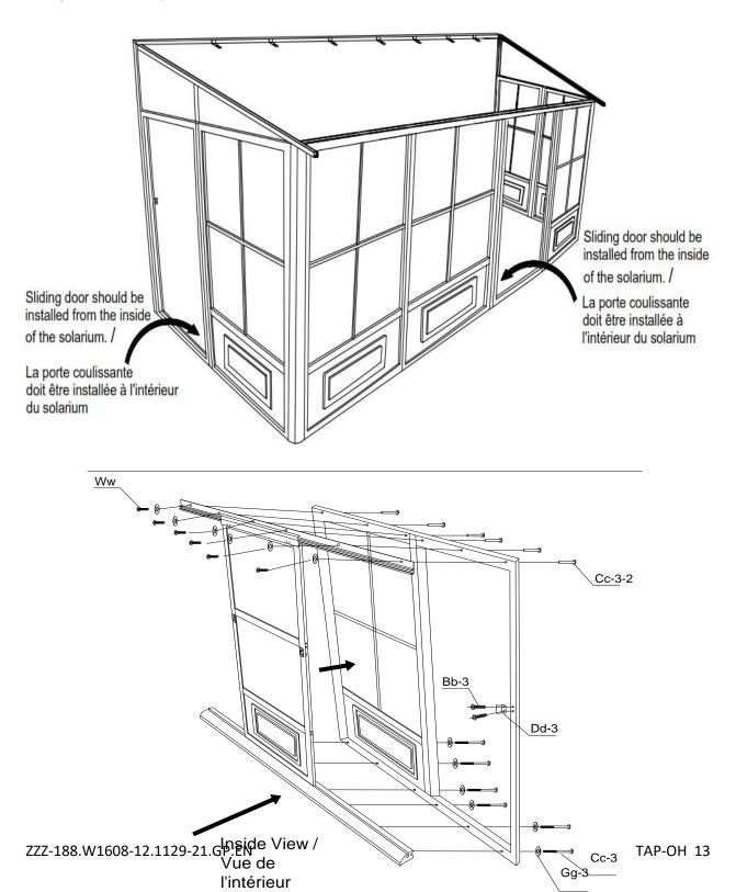
Set U-3 rafters over the middle of each panel with Bb-3 screws at the top and two (2) Z-3 screws over the brackets on frame manually. Set U-3 rafter on each joint and use Z-3 screws manually. Do not use power drill.
