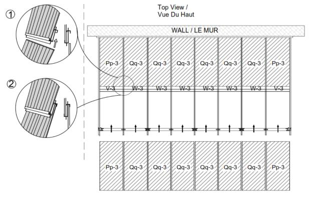
Starting at either end, add X-3 edging and one (1) R-3 bracket and screw with Bb-3 manually, do not use power drill. Add Y-3 edging and repeat until you reach the end, then add the X-3 edging.
