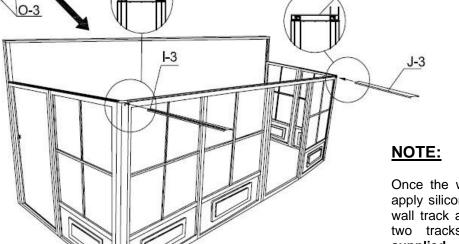
Once the wall track is in place, apply silicon along the top of the wall track and at the joint of the two tracks. Silicone is not supplied.
