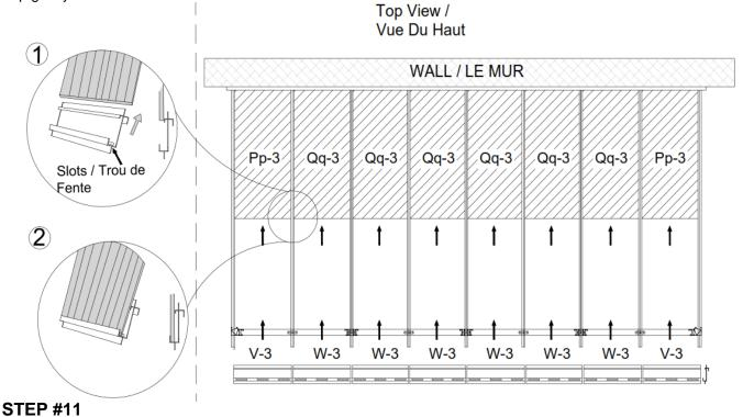
Insert the second row of panels into the lower groove on the rafter. Slide panels until they reach the aluminum pieces between the panels and gently tap on the panel to guide it into the aluminum groove. Use a spatula if needed to make it fit. Insert two (2) Pp-3 on either end, then insert the Qq-3 panels.
