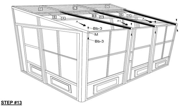
Install crossbeams (L1, L2) under rafters (F, F1, G). Use Cc-3-1 screws + Hh-3 nuts for the splice, then secure to the rafter with Cc-3 screws. Make sure it's tight.
