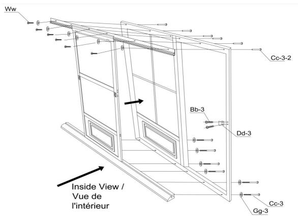
Slide roof panels (A, A1) onto lower track of rafters (F, F1, G).
