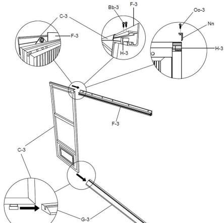
Lift up door and track inside of solarium then set it over the door opening by screwing at the top. First use bolts (Ww) and washers (Gg-3) on the inside and female bolts (Cc-3-2) on the outside for the top assembly. See diagram below. Attach lower track with bolts (Cc-3) and washers (Gg-3). Set up door latch Dd-3 on the side required for your door to lock, adjust latch as required.
