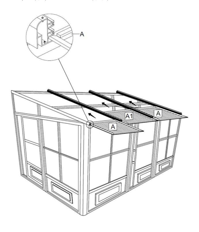
Slide roof panels (B, B1) onto middle track of rafters (F, F1, G).
