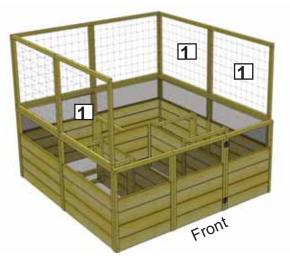
**4.** Position a second **Rear Panel (1) - 46" wide x 33 5/8" high** on top of the rear raised bed frame. Hold both rear deer fence frames together and starting at the top, screw together with **4 - 2 1/2" screws** as shown above. Screw bottom of frame down to raised bed frame with **4 - 2 1/2" screws**. Complete remaining side and rear panels attachments following **Steps 2 and 3**.
