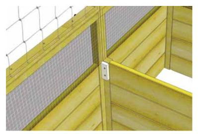
**11.** The **Door Stop (I)** and screws were included with your 8x8 Raised Garden Bed Kit. See **Step 21** of that manual. Install the Door Stop at the top of interior panel frame as shown above.
