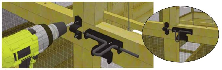
**10.** Attach Black Barrel Bolt to door and panel frame using **6 - 3/4**" **black screws**. Note how female part of Barrel Bolt is positioned higher than male. Do a dry run first to position Barrel Bolt correctly, then attach. Pre-drill with 1/16" drill bit to prevent wood from splitting.
