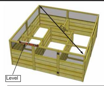
**1.** Prior to installing your Deer Fence Option Kit, confirm your 8x8 Raised Bed is level and square. Measure diagonally inside corner to corner (approximately 128") in both directions. Adjust as required. Use a level to determine if the tops of the bed frames are sloped and adjust if necessary.
