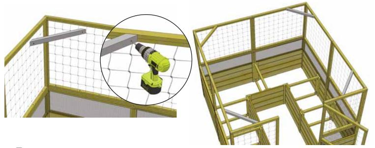
**7.** Attach **Corner Brackets with angle cut ends - (4)** on the inside frames at the top. Use **2 - 2 1/2**" **screws** per bracket. Screw on an angle. Pre-drill ends with 1/16" drill bit to prevent wood splitting.
