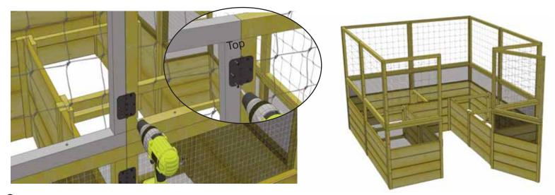
**6.** Locate both **Black Plastic Hinges (3)** and attach to deer fence frame with **6 - 3/4**" **black screws per hinge** as shown above. Use 1/16" drill bit to pilot hole shallow holes before attaching to avoid splitting deer fence framing. Open and close door to check door aligned correctly. Adjust as required.
