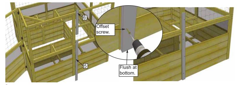
**8.** Locate Vertical Panel Supports - Long (5) - 3/4" x 2 1/2" x 45" and Vertical Panel Supports - Short (6) - 3/4" x 2 1/2" x 22". Starting with 45" long support first, center on panel frames, flush at bottom and attach with 4 - 2" screws. Offset the screw to either side of the support to ensure you contact the heart of the bed frame.
