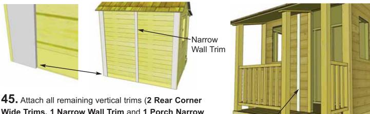
**45.** Attach all remaining vertical trims (**2 Rear Corner Wide Trims**, **1 Narrow Wall Trim** and **1 Porch Narrow Trim**). Use 6 finishing nails per piece to secure. Space Narrow Trims equally on wall seams before attaching.
