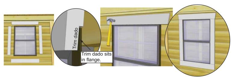
**61.** Position **Window Trim** around window doing a dry run first and attach with **4 - 1 1/2**" **Finishing Nails** per piece. Window trim has a small dado on reverse face. Outside flange of window will roughly sit in the dado to give a better fit.
