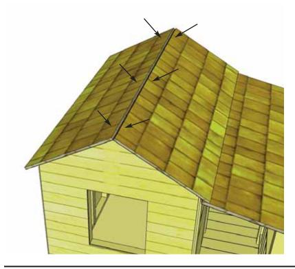
**42.** To complete Roof Section, attach Front and Rear Roof Panels from the top into the Roof Ridge Beam with 3 - 2 1/2" screws per panel.
