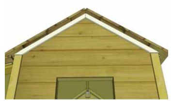
**46.** Position **Side Facia Trims** on ends of roof plywood. Align tight against underside of shingles so both Side Facia Trims meet evenly at the peak. Attach to end of plywood with 4 finishing nails per piece.
