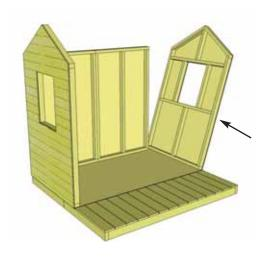
**16.** The top wall framing of both Solid Backwall Panels should also align with each other. With Solid Backwall Panels correctly aligned, attach vertical studs together with 3 - 2 1/2" screws . Locate and position **Right Gable Side Window Wall Panel**.
