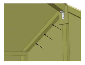
**37.** With Rear Roof Panel evenly positioned on Gable Walls, tack Roof Panel down to framing from the inside with 3 - 2 1/2" screws per side (tack = don't screw completely, roof may need adjusting later).
