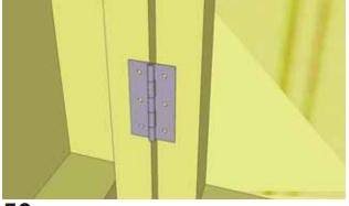
**56.** With Bottom Door correctly positioned, attach **Hinges** to Door Jamb and Door Framing with 3/4" Silver Screws. Before completely securing all screws, check door alignment by opening and closing door. Adjust hinges as necessary.
