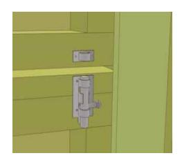
**58.** Attach **Door Handle** with 3/4" Black Screws and **Interior Barrel Bolt** with 3/4" Silver Screws. Handle is positioned on bottom door. Interior Barrel Bolt (silver) to door studs on the inside of Top and Bottom Doors.
