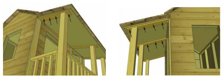
**41.** Using 2" screws, secure Porch Roof Panel to each Porch Rafter from underneath.
