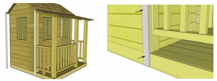
**44.** Attach **Narrow Wall Trims** on both Gable Side Window Wall Panels using 6 finishing nails per piece. Position Narrow Wall Trim so it caps Wide Trim. See **Step 45** for rear detail.
