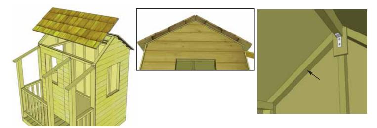
**38.** Position second Roof Panel evenly on front Gable Framing. Tack down with only 2 - 2 1/2" screws. Porch Roof may need to slide under Roof Panel and some play is required before completely securing.
