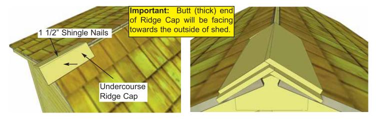
**50.** Place First Roof Ridge Cap on roof peak (Undercourse Cap) overhanging shingles by approximately 1". Attach with 2 - 1 1/2" Shingle Nails. Place 2nd Ridge Cap 1" back from 1st cap.
