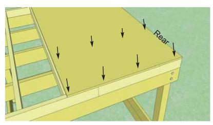
**19.** Locate **Plywood Floor** and position flush with outside of rear Floor Joist Frame. When in correct position, attach with 1 1/4" screws. Use screws every 16".
