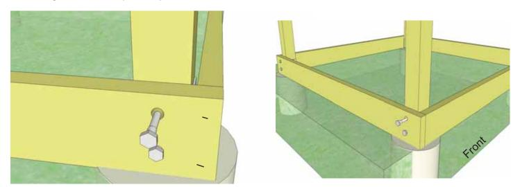
**10.** When correctly leveled and positioned, place **Lag Bolts with Washers** through Pre-Drilled holes of Lower Side Girders and tighten with 9/16th wrench. Complete both Side Girder attachments.
