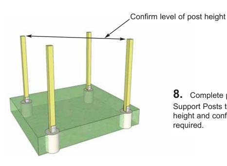
**8.** Complete positioning and attaching all Support Posts to Post Mounts. Measure post height and confirm that it is level. Adjust as required.
