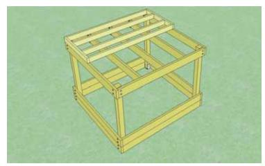
**17.** Carefully lift completed Floor Joist Frames and position on Elevated Platform so long floor joists run perpendicular with interior floor joists of platform.
