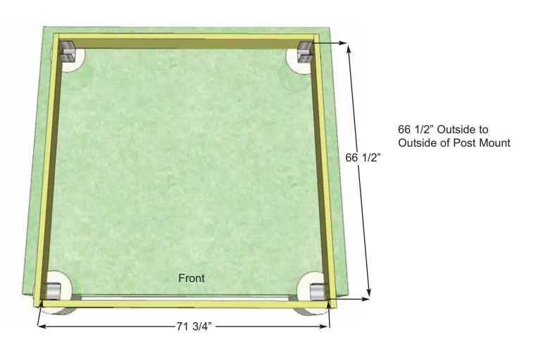
**5.** Complete positioning of all Post Mounts. Measure and confirm that it is level. Adjust as required. Allow concrete form to set as per manufacturer's recommendations.
