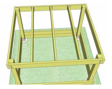
**15.** Complete attachments of remaining Interior Joists.
