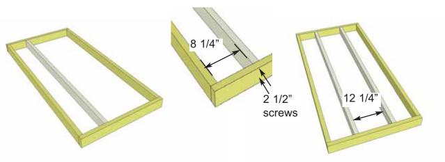
**16.** Next, attach **Floor Joist Frames**. Frames require two interior Floor Joist attachments. Measure Joist (8 1/4") from inside of Floor Joist Frame to inside of Floor Joist and attach with 2 - 2.5" screws per end. Complete attachments of both Floor Joists and both Floor Joist Frames.
