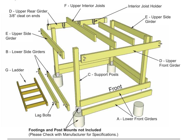
1. Before you receive your Playhouse, clear the construction area. Remove all debris; roots, grass, rocks, etc. Dig holes for **Concrete Forms** (Sonotube). Geographic areas vary for depth and diameter of forms so check with building authority first. Concrete Forms should be dug on 69" centers for the front and 63" for the sides. Confirm front and sides by measuring 93 1/2" diagonally.
