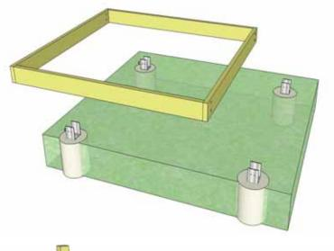
**6.** After Post Mounts are set in the forms, carefully remove Lower Girder Section and place to the side.
