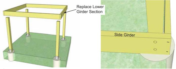
**9.** Carefully lift and re-position Lower Girder Section around Support Posts with your helper. Align Girders as per **Step 4**.
