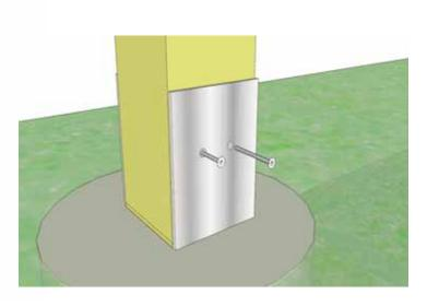
**7.** Locate 3 1/2" x 3 1/2" **Support Posts**. Position and attach bottom to Post Mount. Use Hardware recommended by Post Mount Manufacturer.
