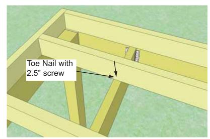
**18.** Align Floor Joist Frames so they sit flush with outside of Upper Girders of Elevated Platform. When positioned correctly, secure Floor Joist Frames with 18 - 2.5" screws, toe nailing on angle into Interior Joists. IMPORTANT: Be careful that no screw tips are exposed after toe nailing. Run hand down Joists and visually inspect before proceeding. Remove and reposition screws if necessary.
