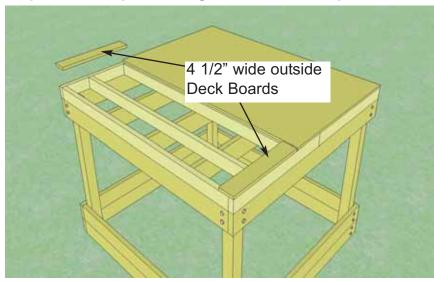
**20.** Locate **Deck Boards** (12 @ 5 3/8" and 2 @ 4 1/2" wide x 3/4" x 24" long). Start by positioning both 4 1/2" wide boards to the outside of Floor Frame.
