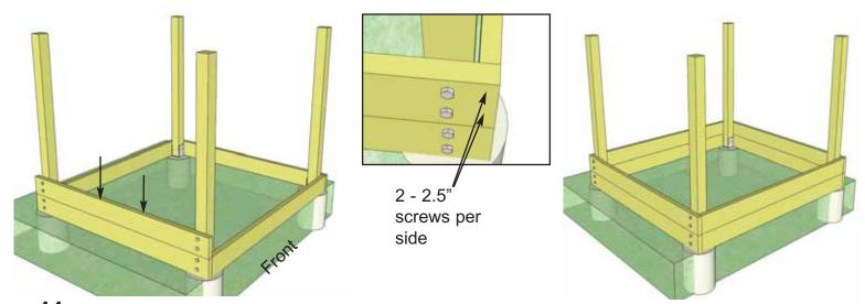
**11.** Place second Left Side Girder between Support Posts directly on top of Lower Girder and attach as per Lower Girder. Attach Front and Rear Girders with 2 - 2.5" screws per side. Complete Right Side Girder to complete as per left side.
