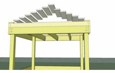
**22.** Position remaining Interior Deck Boards (12 @ 5 3/8" wide) between Outside Deck Boards.
