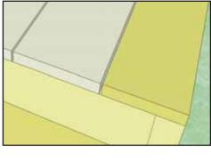
**23.** Space Deck Boards so there is approximately an 1/8" gap between boards and attach with 3 - 1 1/4" screws per piece.
