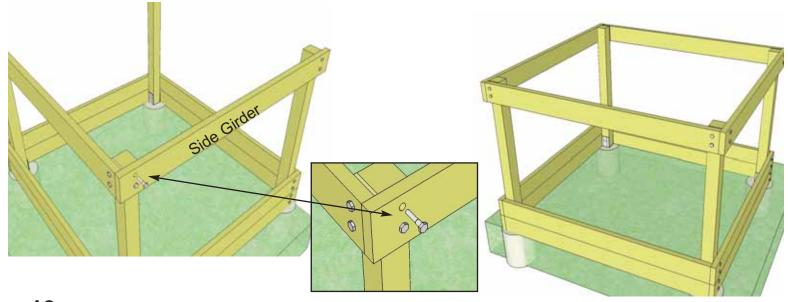
**13.** Locate **Upper Side Girder** (70" long and Pre-Drilled) and attach with Lag Bolts to Support Posts as per **Step 12**. Complete all Upper Girders as Per **Steps 12 & 13**.
