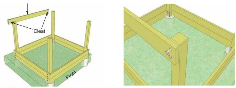
**12.** Locate **Upper Rear Girder** (Pre-Drilled and with a 3/8" Cleat on inside ends). Attach to Support Posts with 4 Lag Bolts. Make sure Girder is flush with top and sides of Posts with Cleat to the inside.
