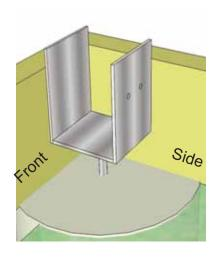
**4.** Place Post Mount in wet Concrete Form and position as illustrated.
