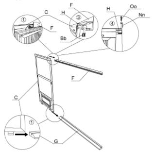
Step 3: Please note the sliding door should be installed from the inside of the solarium.
