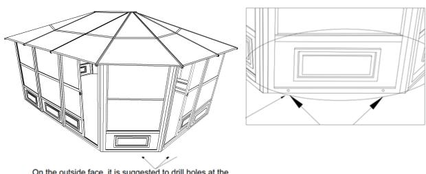
On the outside face, it is suggested to drill holes at the bottom end of the panels to permit drainage when installing on Concrete floor
