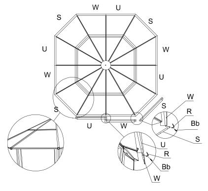
**Step 11:**Use the cross bars (T, V, X) to affix to the roof using bolts (Ff).
