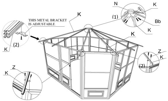
**Note:** Do not tighten the bolts right away as you may have to adjust the angle when inserting the PC roof panels.
