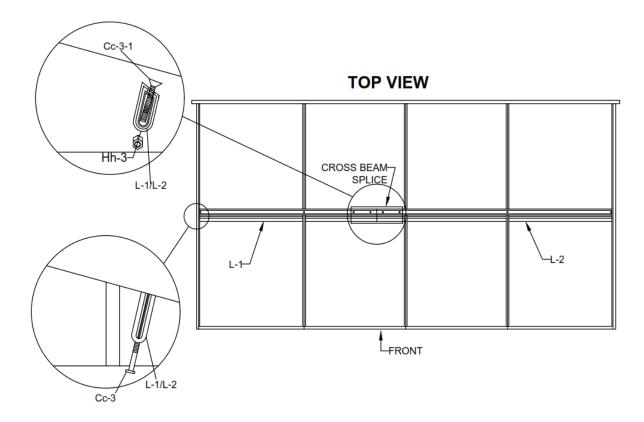
Anchor the solarium to the deck or floor securely using screws and shields supplied.
