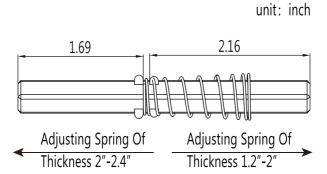
b.Tighten up the 3pcs connection rods to the outside chassis and make the two arrowheads face each other.
