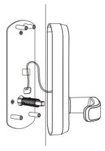
d. Install the inside chassis onto the mounting plate and fasten it with 4pcs  $\rm M4^*12~screws$
