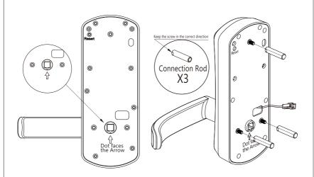
c.Insert the square iron stick smoothly across the latch. Make sure the stick edge slides into the hole on the outside handle. Get the wire on the handle across the space.
