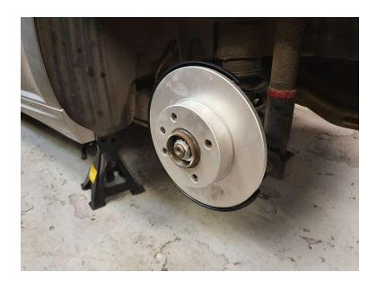
13. From the rear of the hub, fit the caliper carrier using two M8x30 Hex Socket Bolts (Torque Setting 80Nm).
