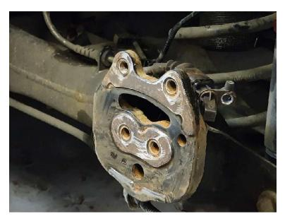
9. Clamp off the body to axle brake flexis and remove the hard brake line connections from the flexis.
