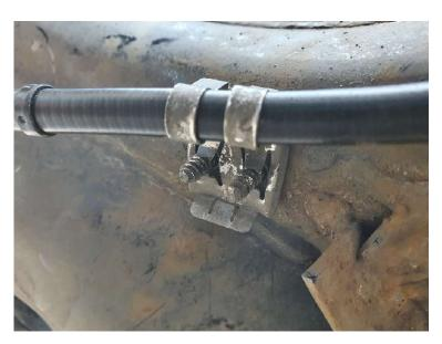
21. Clip the new handbrake cable into the caliper bracket and locate the ball end into the handbrake mechanism lever.
