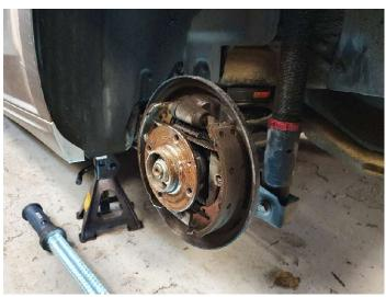
Remove the centre hub nut and slide off the hub bearing assembly.
