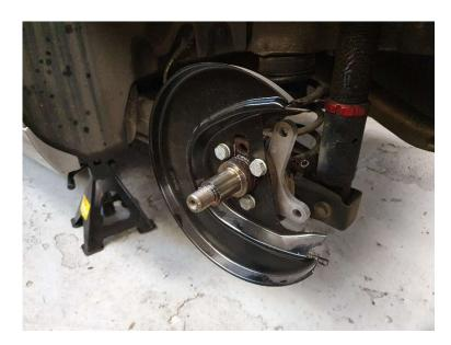
11. Refit the hub bearing assembly and secure using the M20 Stub Bearing Nut (Torque Setting 70Nm plus 30 degrees). Refit the ABS sensor (Torque Setting 8Nm).
