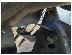
17. Repeat steps 1 to 16 for the opposite side of the vehicle, then bleed the brake system in accordance with the manufacturers' guidelines.
