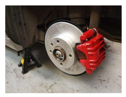
**15.** Secure the banjo end of the new braided caliper brake hose to the caliper (Torque Setting 30Nm).
