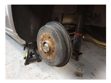
2. Remove the screw securing the rear brake drum, and the brake drum itself.
