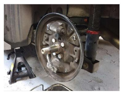
8. Remove the four stub axle bolts and lift away the drum backing plate and stub axle, revealing the 'pig face'. Clean any rust or rough surface off the pig nose, ears, and chin to provide a good surface for the stub axle adaptor plates.
