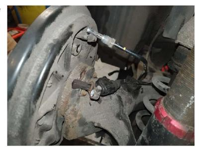
6. Push in and quarter-turn the brake shoe retaining clips/springs and remove.
