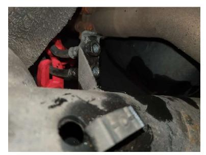
10. Fit the stub axle adaptor, stub axle, and brake dust shield, securing with four M8x40 Hex Socket Bolts (Torque Setting 60Nm).
