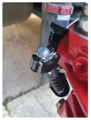
22. Thread the end of the handbrake cable into the guide tube until fully seated. Clip the cable back into the retaining hooks and re-install the retaining clip. It is not essential that the metal ring on the new handbrake cable aligns with the retaining clip.
