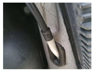
23. Inside the vehicle, locate the end of the handbrake cable into the tensioning bracket. Repeat steps 20 to 22 for the opposite side of the vehicle, then adjust the handbrake for correct operation as per the manufacturers' guidelines. Once completed, reinstall the handbrake cover.
