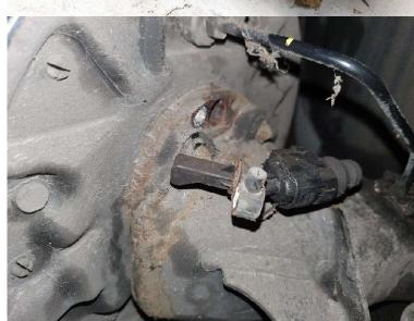
5. Disconnect the drum brake fluid pipe.
