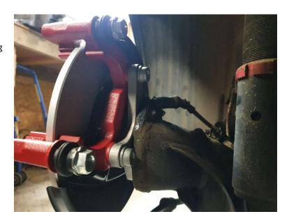
14. Fit the brake pads into the caliper, using copper grease in the appropriate areas, and install the caliper onto the carrier using two M6x22mm Hex Bolts (Torque Setting 35Nm).
