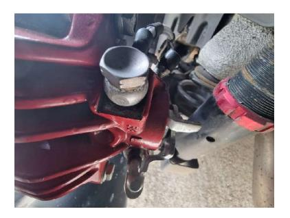
16. You will need to make up new brake lines from the 'body to axle' flexi mounts to the new caliper flexi hoses. Use the existing drum brake lines as templates but terminate each pipe in a flare fitting just after the kick-up either side after the plastic retaining bracket.
