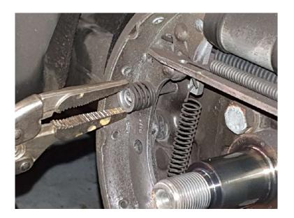
7. Remove the brake shoe assembly and disconnect the handbrake cable.
