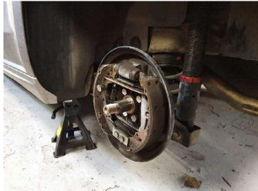
4. At the rear of the drum assembly, remove the ABS sensor retaining bolt, and the sensor itself.
