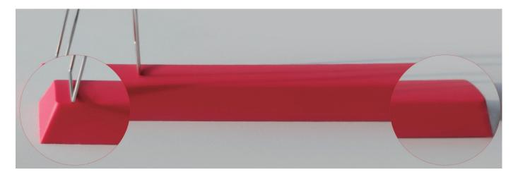
2. Stress marks on the sides of the keycaps may be present, which can be more noticeable in darker colors and under different lighting conditions.
