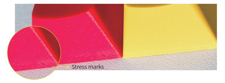
3. The front of the keycaps is free of any defects, and any side defects  $\leq$  0.3mm<sup>2</sup> are within the acceptable range of our quality inspection.
