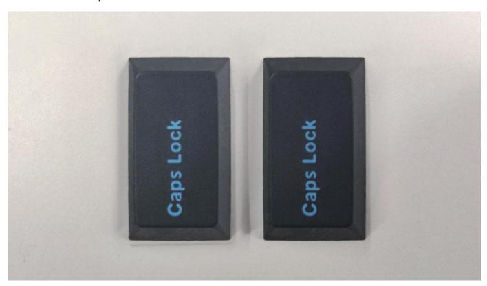
6. There might be a slight burr on the edge of the keycap, but this will not be visible from the front after installation and should not affect the appearance or function of the keycap.
