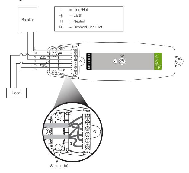
Note: All outside wire diameters must be the same and must be between 5.2 mm to 8.5 mm (0.2 in to 0.33 in)
