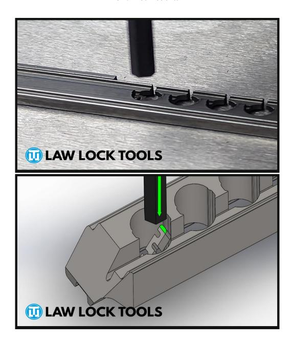
Now using the Allen key continue to push the pin from the upper edge (highlighted green above) of the pin straight down into the final position in the hole.
