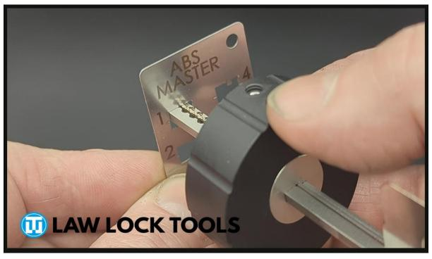
It is also possible to use the key decoder card to set the impressioning pins to a known code and use the tool as a MUK (Make Up Key) Just be sure to keep the card centred and at a level 90 degree to the impressioning pins so as not to dislodge them if you pushed from one side etc.
