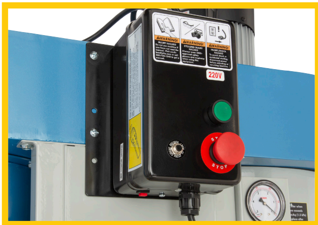
The powered control box with remote pairing reset button and thermally protected magnetic switch
