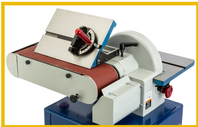
The belt sanding fence with heavy-duty miter gauge
