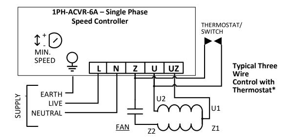
An external thermostat or switch can be fitted to enable the fan to run at a pre-set speed adjusted by the controller and a maximum speed set by temperature of the thermostat or operation of the switch. Connect the thermostat or switch to the U and Z of the controller as shown in the circuit diagram.
