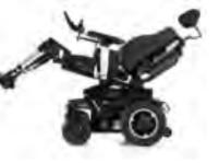
Powered elevating leg rest (ELR)
