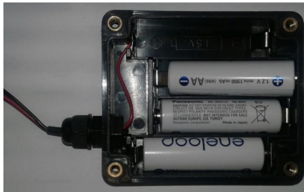
Replacing battery in battery box
