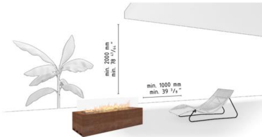
Figure 1: Minimum distance to flammable materials
