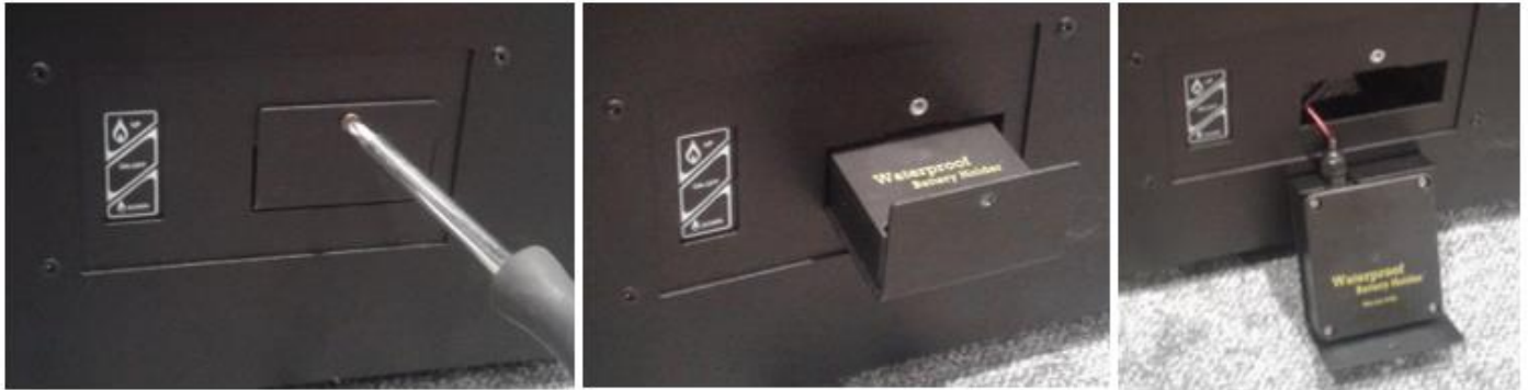
Photo 6: Removing of the battery container
