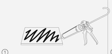
Apply adhesive evenly on the tile and stick it directly to the wall. You can use a level if necessary.
