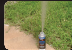
Aerosol Grenade Vertical Deployment & Distribution Pattern
