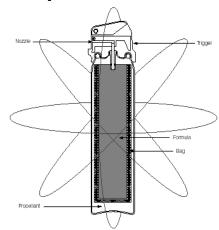
SABRE CFT<sup>®</sup> units operate in any orientation, in any plane continuously, giving officers greater ability to fire OC in any situation.
