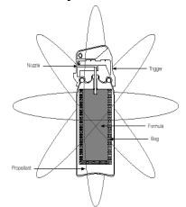
SABRE CFT® units operate in any orientation, in any plane continuously, giving officers greater ability to fire OC in any situation.
