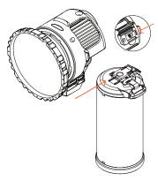
Push light onto battery until it "clicks" **Tip:** Push from the front top of the optic
