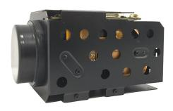
Network zoom camera module is a fully integrated network block camera including Image sensor, long range zoom lens, video encoding, video analysis and network transmission functions. It is designed to be flexible embedded into PTZ cameras, bullet cameras, Pan/Tilt positioning cameras, AGV robot systems, UAV drones, etc. Linovision network zoom camera modules provide standard 36-pin cable and complete SDK/ISAPI protocols. It comes with intuitive WEB GUI and CMS software, and OEM is welcomed.
