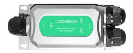
POE-EXT6002GP is a Gigabit IP67 waterproof PoE extender independently developed by our company. It supports one RJ45 (PD) port in and 90W input (IEEE802.3bt). Two ports have PSE function, Port1 up to 30W, Port2 up to 60W, without configuration, plug and play.
