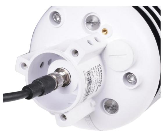
When using the device with a heating function, a separate 24V (24V@1A is recommended) power supply is required. Gray wire #5 is connected to the negative of the power supply, and pink wire #6 is connected to the positive pole of the power supply.
