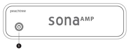
Standby Switch: After turning the sonaAMP on with the AC Power switch on the back panel, this button will allow you to switch between "on" (blue light) and "standby" (red light). Standby draws very little power so we suggest leaving the amplifier on from the back panel and using this switch for daily operations.
