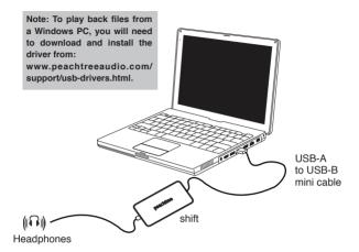
Using the supplied USB-A to USB-B mini cable, connect the USB-B mini connector to shift and the USB-A connector to the PC.
