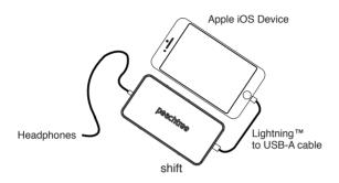
Using the supplied Lightning™ to USB-A cable, connect the USB-A connector to shift and the Lightning connector to the iOS device
