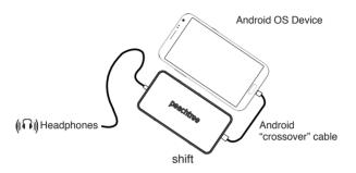
Using the supplied Android "crossover" cable, connect the USB-B mini connector to shift and the USB-B micro connector to the Android device
