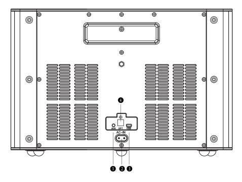
AUX Analog Audio Input: Accepts line-level analog input from a tuner, cassette deck, phono preamp or other type of <u>line-level</u> analog source.
