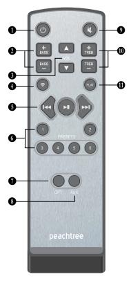
On/Standby Button: With the AC power cord connected, this button toggles the unit between On mode (which selects the last input used) and Standby mode which lights the LED red. Note: the input LEDs will flash white in a sequence when the unit goes into on or standby mode.
