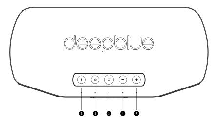
Bluetooth: Push and release to select the Bluetooth input. The LED will light blue for 10 seconds indicating the input is selected. Push and hold for 5 seconds to enter Bluetooth pairing mode. The Bluetooth LED will flash blue and white in this mode. Enter the Bluetooth menu on your device and select "deepblue<sup>3</sup>" to confirm the pairing. The Bluetooth LED will light solid blue and you will hear a double-beep when the deepblue<sup>3</sup> is connected to a Bluetooth device.
