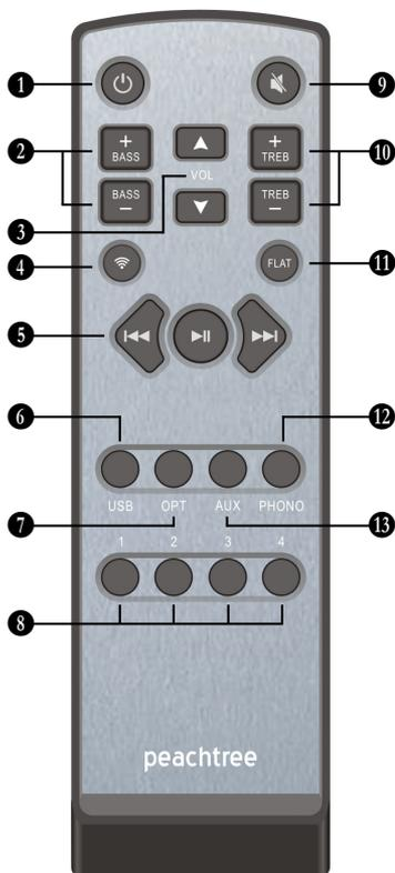
**1 On/Standby Button:** With the AC power cord connected, this button toggles the unit between On mode (which selects the last input used) and Standby mode which lights the LED red. Note: the input LEDs will flash white in a sequence when the unit goes into on or standby mode.
