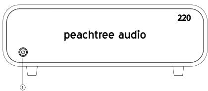
Standby Switch: After turning the Peachtree220 on with the AC Power switch on the back panel, this button will allow you to switch between "on" (blue light) and "standby" (green light). Standby draws very little power so we suggest leaving the amplifier on from the back panel and using this switch for daily operations.
